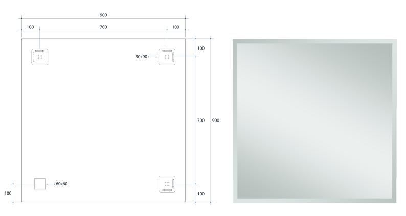
Note: All dimensions are in millimetres (mm)
