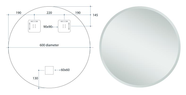
Note: All dimensions are in millimetres (mm)
