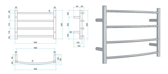
This rail has Multiflex wiring which means that there is a connection point on both the left and right hand side of the rail and the lead can be connected to either side. Being a dry electric element rail, this can be mounted either way up meaning the wiring can be from any of the four mounting points.
