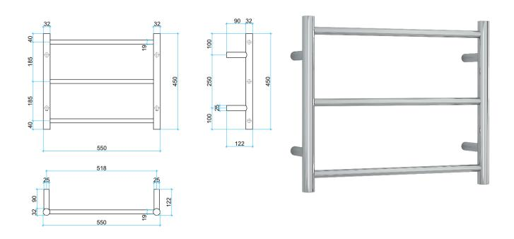
This rail has Multiflex wiring which means that there is a connection point on both the left and right hand side of the rail and the lead can be connected to either side. Being a dry electric element rail, this can be mounted either way up meaning the wiring can be from any of the four mounting points.
