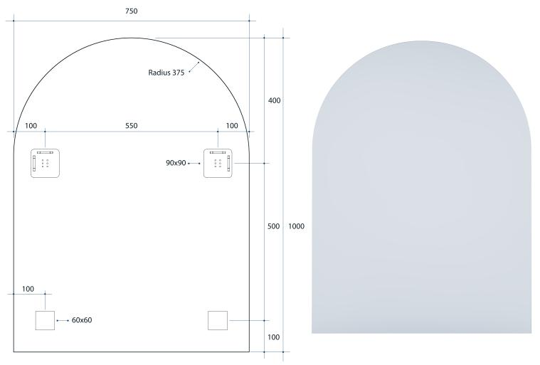
Note: All dimensions are in millimetres (mm)
